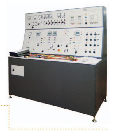
circulating current and distance numerical protection. It also covers relay setting and tripping characteristics, as well as grading and discrimination under fault conditions.
